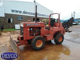
**Ditch Witch 6510DD Trencher w/ Deutz Motor**
