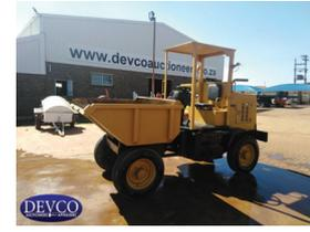
**1m³ Concrete Dumper Truck**
